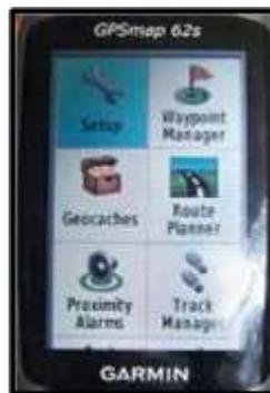
**Figure 12: SETUP menu of the GPS 62s**
