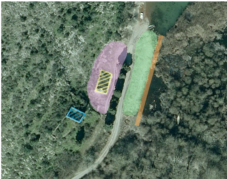
Picture 3 - blue square is the house used by PENP, yellow square is the collapsed military object which will be removed, orange line is the surface of the cleaned water channel, green surface is the future parking spot and pink surface is the future camping spot.
