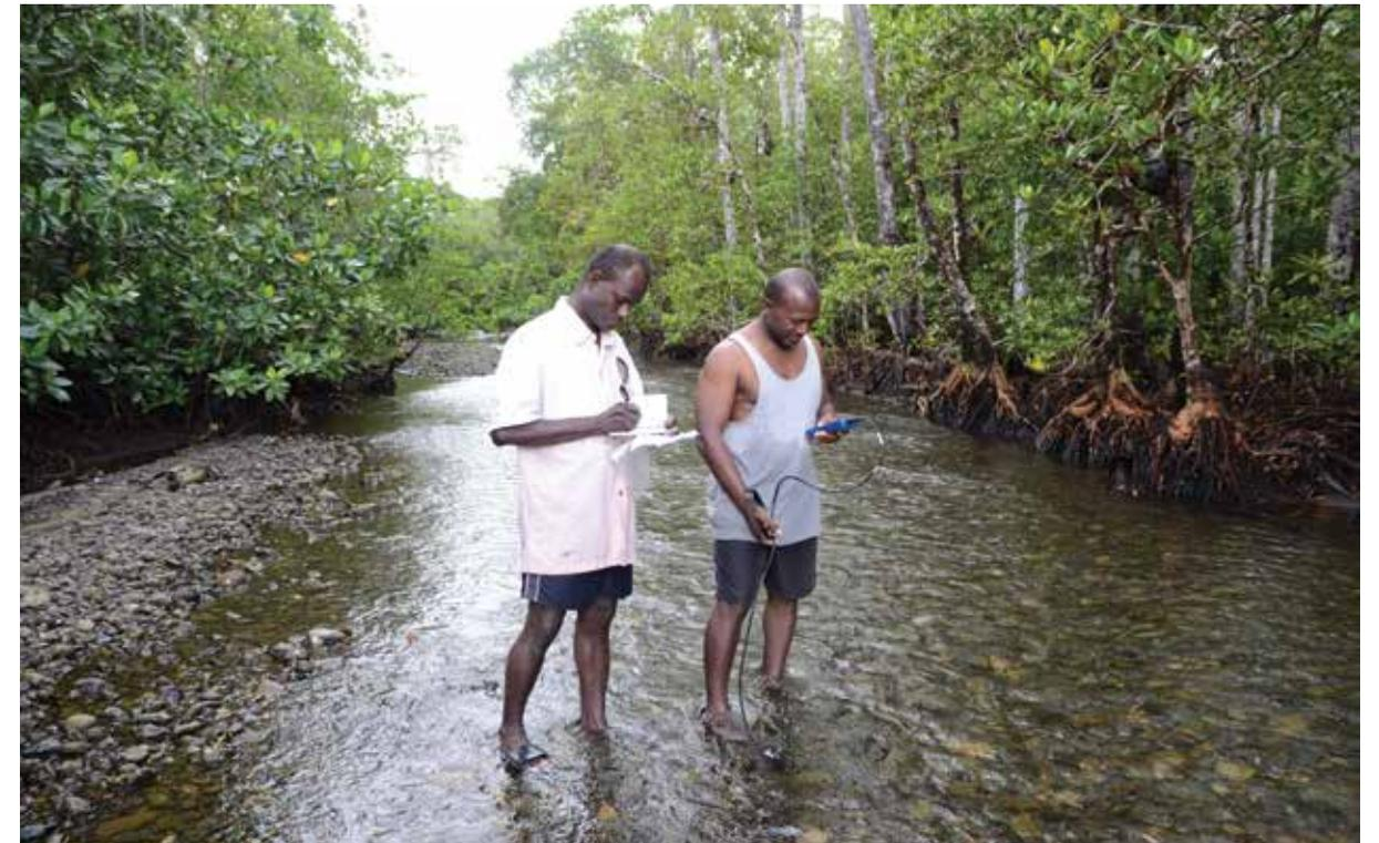
*Collecting water parameters (conductivity, pH, etc) using a hand held meter, as well as recording riparian vegetation during freshwater surveys.*
