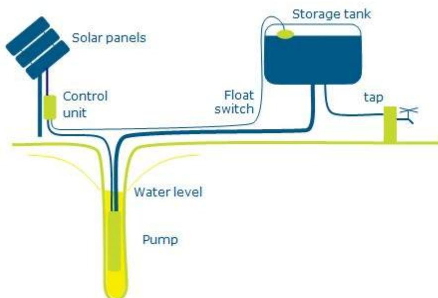
**Figure 2:** Solar pump system layout. PicoSol website.
