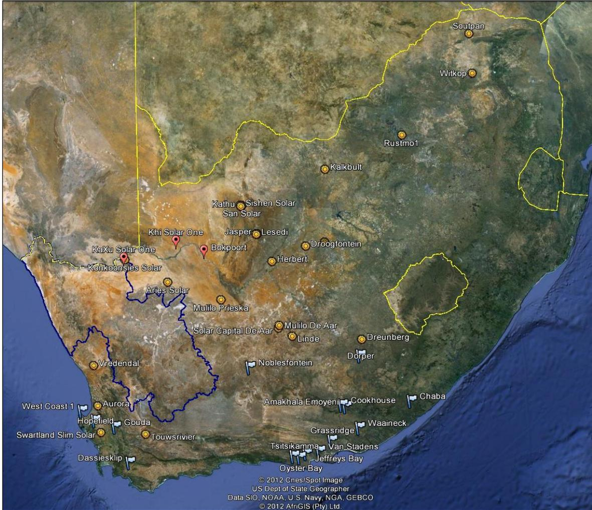
**Figure 1.** Map of the preferred bidders from round 1 and 2 of the Renewable Energy IPP Procurement Program. Wind energy facilities are indicated by the blue flags, solar PV facilities by the suns and CSP facilities by the red markers.
