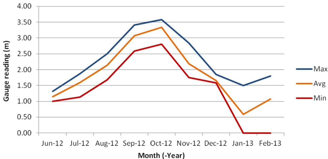
Figure 4. Maximum, average and minimum water levels in canal 90, BPL, per month from June 2012 to February 2013 (note: water level readings are not in meters above sea level due to the absence of benchmarked figures in the area; readings were taken once a day at variable times; the gauge was not placed deep enough to record minimum water levels in January and February 2013).
