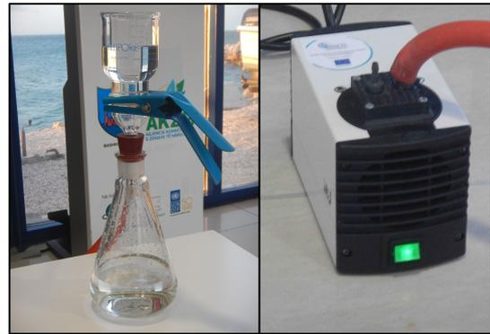
Fig. 5 Water samples filtration system
